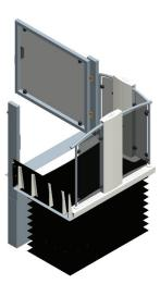
CLEARANCE EITHER SIDE OF STEPLIFT MUST BE <10mm OR >150mm TO COMPLY WITH BS6440.
