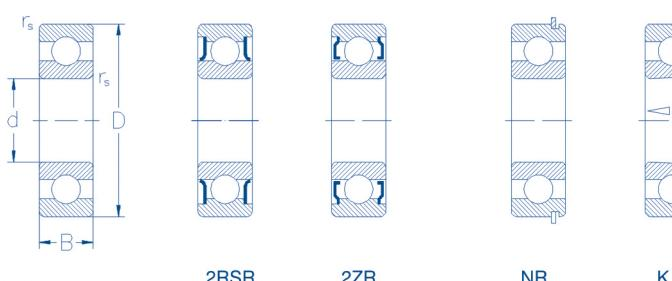
The single-row deep groove ball bearings are available in a wide variety of size and design. Single-row deep groove ball bearings are the most popular type of all rolling bearings. They are non-separable, suitable for high and very high speed applications and they require little maintenance.
