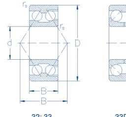
Angular contact ball bearings are non-separable and are designed to accommodate radial and axial loads. They can carry the axial loads in one direction only. For this reason, they are often mounted in pair. The angular contact ball bearings are suitable for high speed applications.
