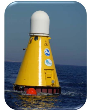
OCB buoy deployed off coast Cyprus
