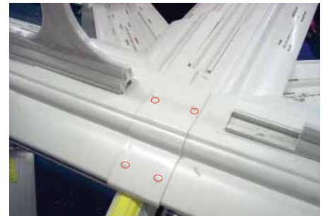
Seal and rivet the rear joint cover to the previous covers completing the joint. Remove excess sealant ensuring the edges of all joint lines are sealed.
