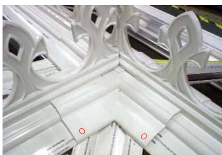
The adjacent line of creasting can now be slid into place over the joint.
