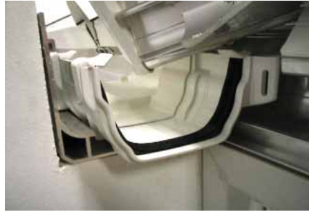
Slide the union over the adapter making sure the union gasket remains in situ.
