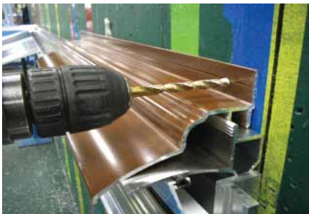
An extrusion line has been incorporated along the back upstand of the aluminium wallplate top cap for the positioning of the fixing screws.
