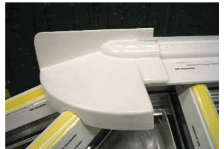
Bay and hip-ended lean to roofs require a radius end top cap. This should be sealed and secured to the wallplate top cap with the plastic rivets supplied.
