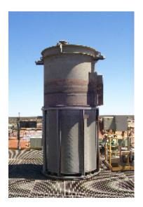
The screens will also become pegged with near sized carbon and other material such as small rocks and need to be removed and cleaned/replaced regularly to prevent tank overflows.
