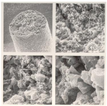
Pictures taken with a microscope showing the porous internal structure of carbon.
