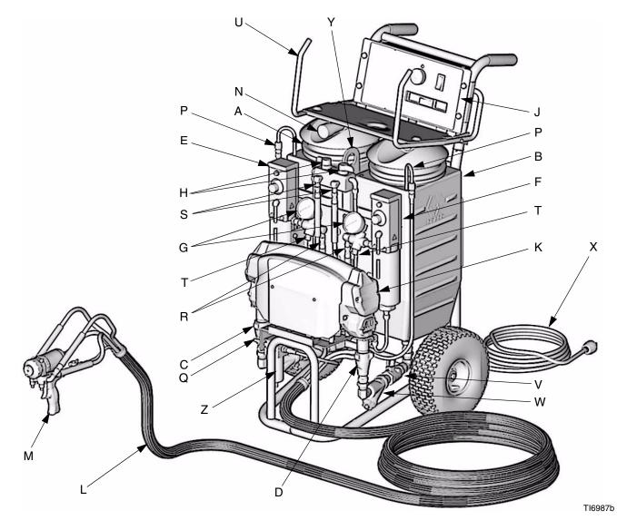
FIG. 1: Component Identification, Heated Packages (Part No. 249804 Shown)
