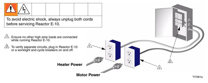
FIG. 5. Use Two Separate Circuits for Two Cord Models
