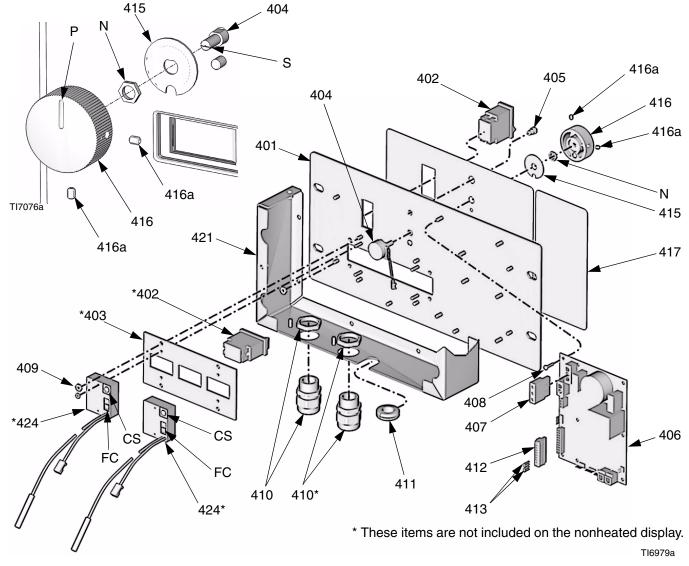
FIG. 11. Control Module (Heated Model Shown)
