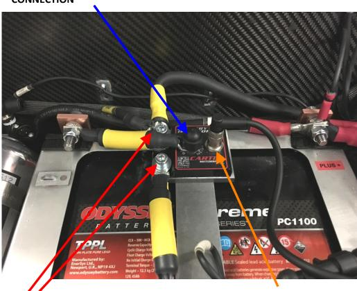
ADDITIONAL EARTH CABLES WHEN NOT MOUNTED DIRECTLY TO CHASSIS
