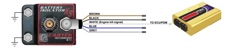
It is also possible to use the Engine Kill Signal to control an Engine Relay/DME. Please check the manufacturers specification before installing.
