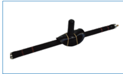
Packer and bladder for the lateral junction repair
