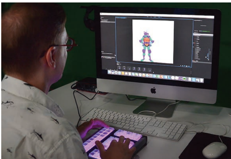
Bringing a Turtle to life requires Adobe Character Animator streaming into the Unreal Engine via NDI in real time.
