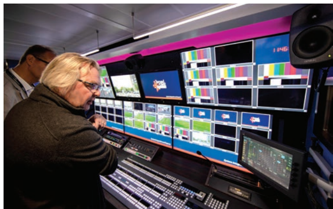
With a need to produce the Polish football league in 4K/UHD HDR, Polish broadcaster Ekstraklasa Live Park has tasked Broadcast Solutions to design an OB van that is able to accommodate 4K/UHD HDR and HD SDR signal workflows.
