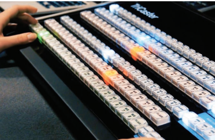
Using NewTek TriCaster allows live editing between animation and live action angles and ISO-recording of all feeds as well as outputting the programme feed to a thumb drive for sharing.
