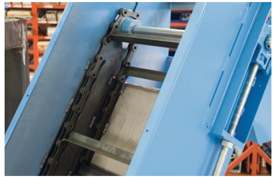
Scraper conveyors: view of lateral chains and carriers
