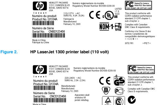
Figure 3. HP LaserJet 1300 printer label (220 volt)
