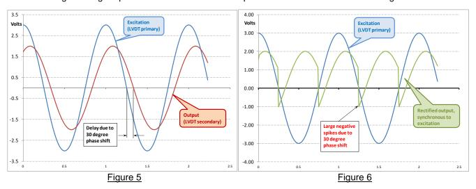
The spikes generated by a large phase shift are difficult to filter (noise level is increased) and more aggressive filtering results in a lower frequency response.
