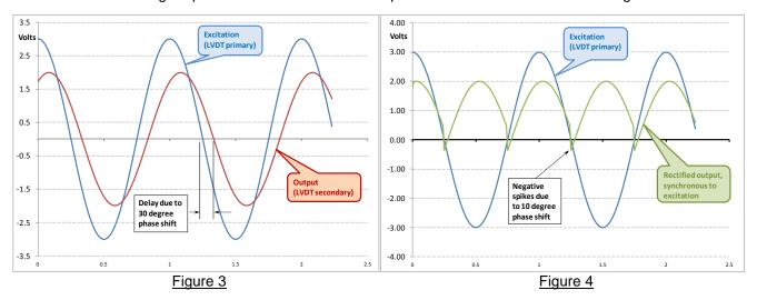
Effect of a large 30 degree phase shift between LVDT output and excitation on the rectified signal:
