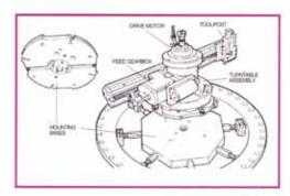
The Silk AX1445 is constructed, as the rest of the range, from the highest quality materials. It is designed to give machine shop accuracy, combined with ease of handling and portability in the flange range of 355mm (14") to 1140mm (45"). The machine consists of four main assemblies:
