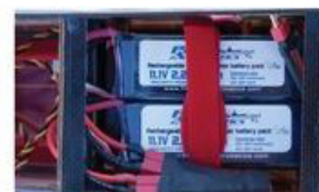
Two 2100 3-cell packs are cheap and provide good flight times. I used genuine Deans Ultra plugs and Wet Noodle Wire to make a custom series adapter.
