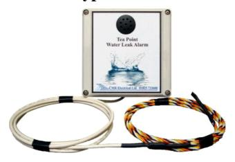
The unit has been designed to be mains powered and give an audible warning when it detects the presents of water or any conductive liquid. Applications for the unit include washing machines, small water tanks, drip trays, sump tanks or high/low level detection, to detect leaks along pipe runs or under.
