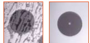
Microphotographs of fiber optic end-faces. Left: a connector carrying fingerprint oils. Right: a clean connector that will transmit data perfectly. Enlarged approx. 200x.
