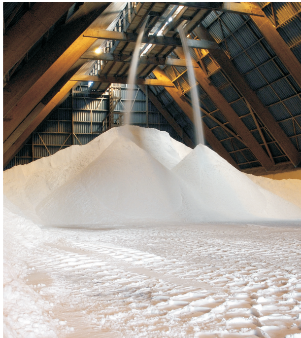
Figure 4 Salt (sodium chloride) is being transferred to a large silo for storage, prior to being converted to chlorine and sodium hydroxide.
