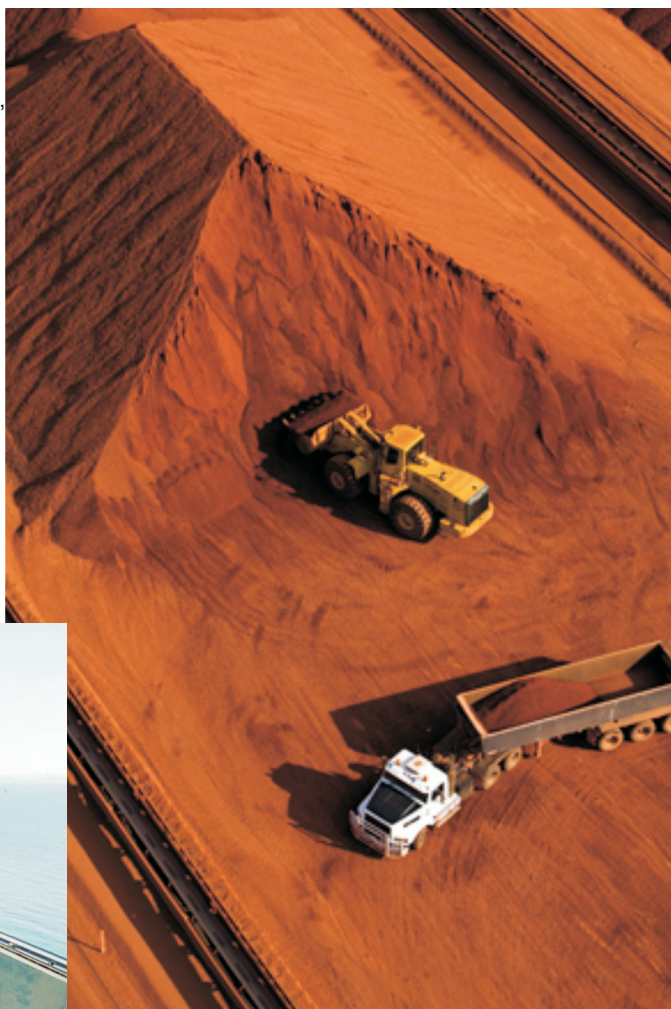
Figure 1 Sodium hydroxide is used in the purification of the ore, bauxite, prior to it being used to make aluminium (Unit 69). This picture shows stockpiling of recently mined bauxite ore at the Gove refinery in the Northern Territory, Australia.
