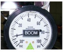
A negative reading pressure gauge is a must in order to know if your suck back is working or not
