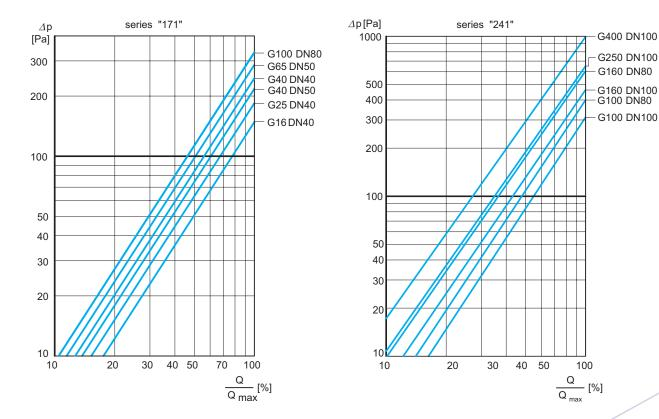
fig. 6 Diagram of pressure loss related to  $\rho = 1,2 \text{ kg/m}^3$
