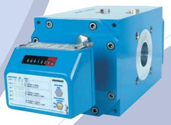
The rotary gas meters are positive displacement meters, designed to measure quantity of gas, for custody transfer or technical measurement applications. The devices are mainly applied for gas flow ranges from 0.2 up to 650 m<sup>3</sup>/h, and the pressure range up to 20 bar. Special design rotary gas meters may also be used in higher pressure installations.
