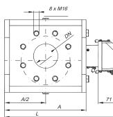
fig.5 Dimensions of the CGR Rotary Gas Meters
