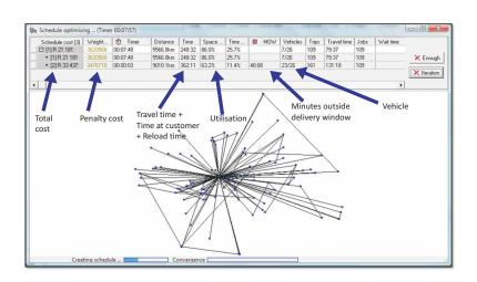
PLATO.Scheduler provides visual feedback as it optimises vehicle trips, clearly showing the number and efficiency of solutions as it works.
