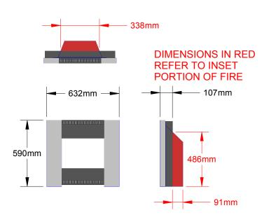
**Hearths** - For hearth mounting (or if the fire is less than 200mm above the ground) then the hearth must protrude at least 100mm in front of the fire and 50mm to either side. A minimum hearth of 732mm wide x 207mm deep is required; the hearth must be a minimum of 12mm thick and be of a non combustible material. The surface on which the appliance is to stand must be flat, level and square to the back panel. Failure to observe this could result in the appliance leaning away from fireplace.
