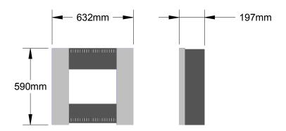
**Hearths** - For hearth mounting (or if the fire is less than 200mm above the ground) then the hearth must protrude at least 100mm in front of the fire and 50mm to either side. A minimum hearth of 732mm wide x 300mm deep is required; the hearth must be a minimum of 12mm thick and be of a non combustible material. The surface on which the appliance is to stand must be flat, level and square to the back panel. Failure to observe this could result in the appliance leaning away from the fireplace.
