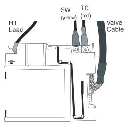
Fit four AA (1.5V) batteries into the receiver unit and the PP3 (9V) battery into the transmitter (hand set). Connect HT lead to receiver & terminal on the pilot assembly. Fold the heat shield as per folding instructions supplied and position it over the receiver.
