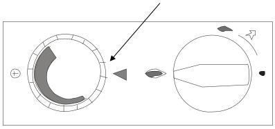
**1.3** To turn the fire off, rotate the right-hand knob fully clockwise back to its OFF position.
