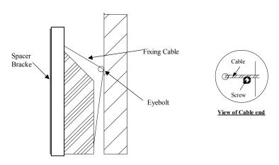
is permissible just to use 2 holes in the wall brackets or to drill through the appliance base and screw it to the floor.
