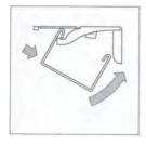
Open the swivel arm fully. Clip the front of the blind headrail over the bracket and then push the headrail up. Finally push the swivel arm backwards as far as it will go.
