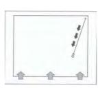
To lift the blind, pull the cord to the left and downwards.
