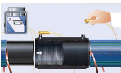
Fig 6-20: Welding in accordance with DVS 2207, Part 1
