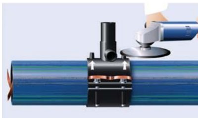
Fig 6-48: Removing the projecting wrap connectors with a suitable tool
