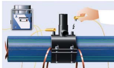
Fig 6-46: Welding in accordance with DVS 2207, Part 1
