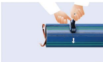
Fig 6-18: Removal of the protective coating with the egeplast M10 peeling tool
