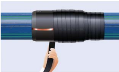
Fig 6-23: Wrapping the weld fitting with Densolen Tape AS 40
