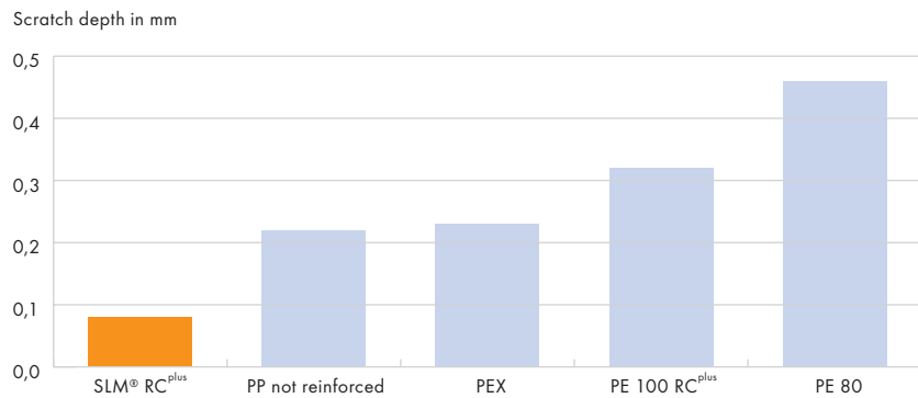
Fig 6-10: Results of scratch testing, official materials testing institute at the University of Hanover
