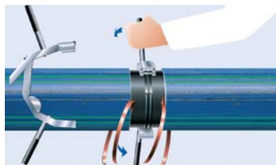
Fig 6-32: Removing of the weld bead with an external bead remover
