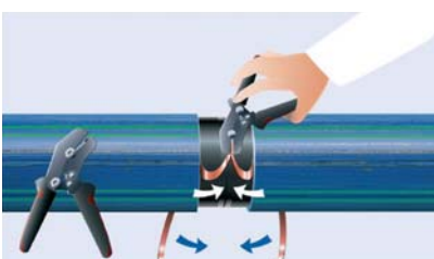
Fig 6-33: Removing the conductive strip coatings and connecting using the egeplast DCT hand riveter
