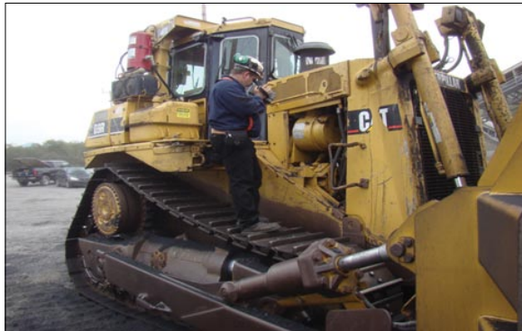
A Thermographer checks engine components such as exhaust ports, the turbo charger, accessory drives, fuel systems and heat exchangers.
