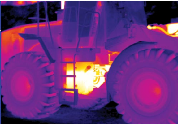
On a front end loader one can use IR to analyze fluid levels, pivot bearings, U-Joints and final drives.
