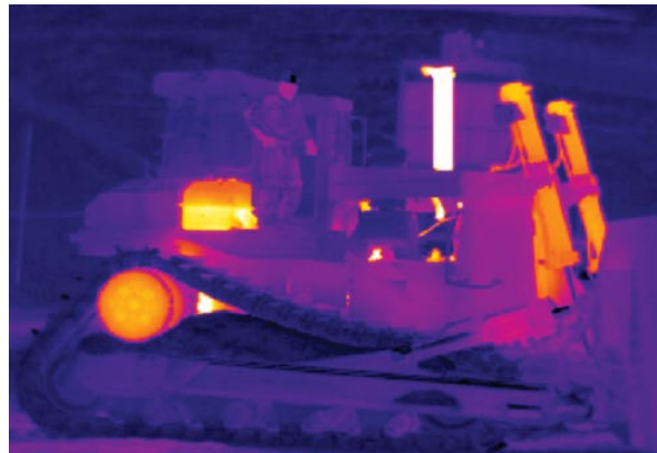
Infrared can help check fluid levels, final drives, and carrying rollers on a bulldozer.
