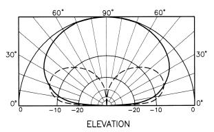
Horizontal GAIN: 4.7dBi Free Space GAIN: -0.3dBi ------ Vertical GAIN: -1.3dBi Height: 30m
