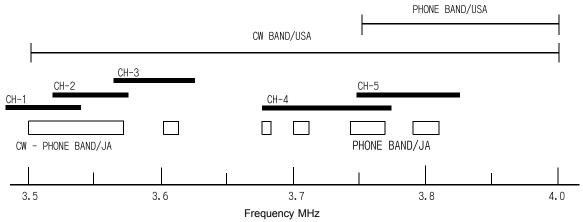
5-CH Coupler, Operation Channel (CD78-L Typical, Bandwidth at VSWR Less Than 2:1)
