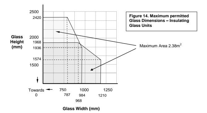
\* The frame section size must be increased to accommodate the additional width of the IGU. Where the IGU includes laminated glass, this must be positioned on the known fire risk side only. If a known fire exposure direction cannot be established then IGUs may not incorporate laminated glass.
