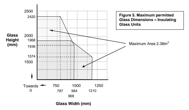
\* The frame section size must be increased to accommodate the additional width of the IGU. Where the IGU includes laminated glass, this must be positioned on the known fire risk side only. If a known fire exposure direction cannot be established then IGUs may not incorporate laminated glass.
