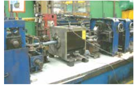
Eddy current tester on small pipe mill
