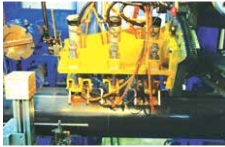
Ultrasonic tester on 16" pipe mill
