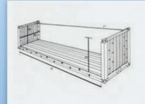
Flat Rack 20' Flat Rack 40' **Inside Length:** 19'4 5.89 m 39'5" 12.01 m Inside Width: 7'7" 2.31 m 7'8" 2.33 m Inside Height: 7'8" 2.33 m 7'8" 2.33 m **Door Width:** 7'6" 2.28 m 7'8" 2.33 m **Door Height:** 7'2" 2.18 m 7'5" 2.26 m Capacity: 32.16 m<sup>3</sup> 66.54 m<sup>3</sup> 1,136 ft3 2,350 ft3 **Tare Weight:** 5,280 lb 2,394 kg 8,490 lb 3,850 kg
