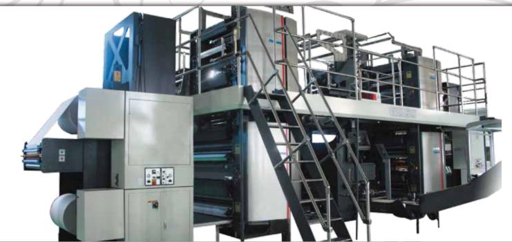
Speed Up to 80,000 cph Cut off 546mm\*914mm
