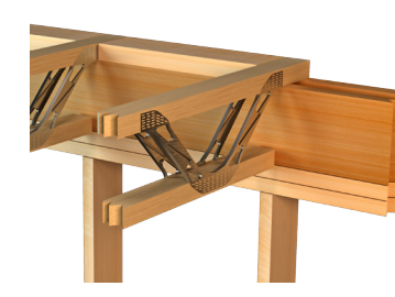
TF5 - Top Chord Support on Standard Panel with Rim Boards - External Wall
