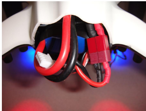
Fig. 7: Stowing of Battery Cables
