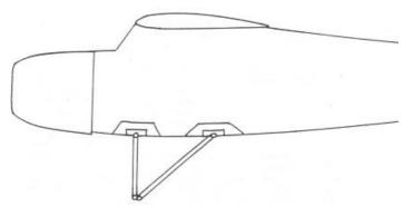
Like the trunnion block gear, this type also flexes out. Smaller diameter wire can be used than with the torsion bar landing gear of the wing. Use 1/8", 5/32", or 3/16" (for big planes), in wing torsion bar gear while 3/32" or 1/8" will work with this type of fuselage gear.
