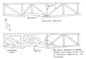
Many kits use a very poor design for fuselage construction.
