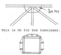
and you want to make it bulletproof, take 1/64" ply and gusset the inside of all joints. It adds hardly anything to the weight, but adds a tremendous amount of strength.
