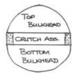
All the bulkheads are glued to this. Cut the bulkheads in half, glue all the bottom (or top) halves in place. Then you can set your wing saddle arrangement and stringers. Take it off the board, add the other side's pieces to finish it off.
