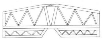
If you're worried about having the lumps showing through the covering, you can use a combination of these two. Put in the needed ribs and put in 1/8" x 1/16" diagonals that don't touch the covering.
