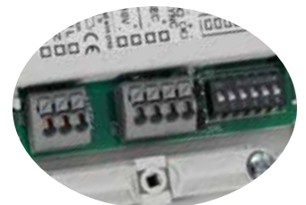
Terminals and dip-switch selection
