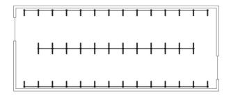
**B.** Snap a chalk line establishing the front edge of the upright bases. The chalk line should run the entire length of the row of rack.
