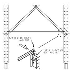
**D.** Now the balance of the uprights can be erected to complete the run. The uprights can be stood either one at a time or in groups of 2.
