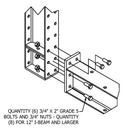
**C.** Mark the arm elevations on the uprights. The marks should be below the top of the arm end plate so as not to show after the arm is bolted in place.
