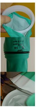
4. secure the glove/cuff assembly 1" (25mm) with white stretch tape. Ensure the tape is evenly applied, pulling gently but consistently, without creases or air bubbles.
