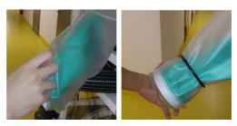
7. Pull the sleeve so that all twists/creases are removed from the sleeve, with your hand in the glove to be fitted, orientate the glove to the required position.
