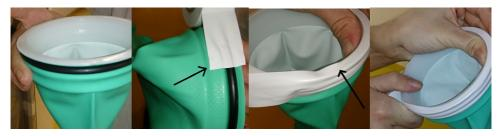
5. Insert a completed glove assembly into the sleeve opening of the isolator. Ensure a left-hand glove is fitted to a left-hand sleeve and so on.
