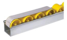
The brake plate made of spring steel brakes the goods on a friction basis using four 33 mm pitch rollers. There is no restarting.
