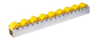
The guide rail, which is particularly sturdy, has a profile width of 1.5 mm and the steel axes are reinforced from 3 mm to 5 mm, which means that they can bear containers weighing up to 80 kg.
