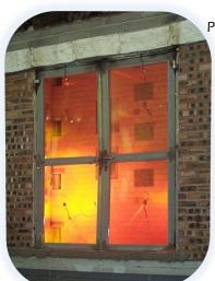
Profiles are produced from 2mm cold rolled pre galvanized steel and filled with a unique fire infill to form the selection of profiles available.
