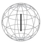
Figure 7: Isotropic Radiation Pattern
