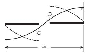
Figure 1: A Half-Wave Dipole Antenna
