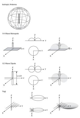
Figure 5: Example Radiation Patterns
