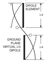
Figure 2: A Quarter-Wave Monopole Antenna
