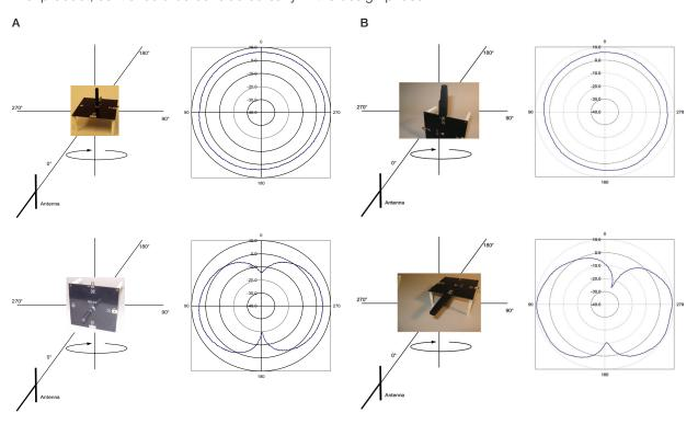
Figure 11: A 418MHz Antenna Radiation Pattern on a 4" x 4" Ground Plane (A) Centered, (B) Edge Mounted
