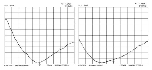
Figure 10: A 916MHz Antenna VSWR on (A) a 4" x 4" Ground Plane and (B) on a 26.5" x 26.5" Ground Plane
