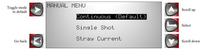
The ExLRT will automatically highlight the mode that has been set to default. The above screen shot shows that the ExLRT default is set to continuous
