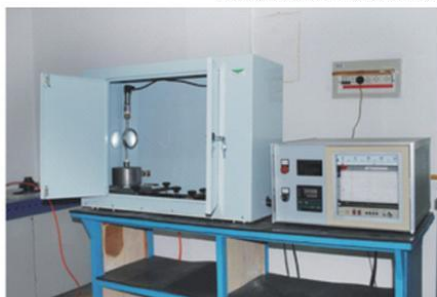
钢丝绳芯胶带渗透性试验机 STEEL WIRE ROPE CORE BELT PERMEABILITY TESTING MACHINE
