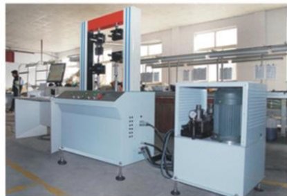
钢丝绳芯胶带动态粘合强度试验机 STEEL WIRE ROPE CORE BELT DYNAMIC ADHESION STRENGTH TESTING MACHINE
