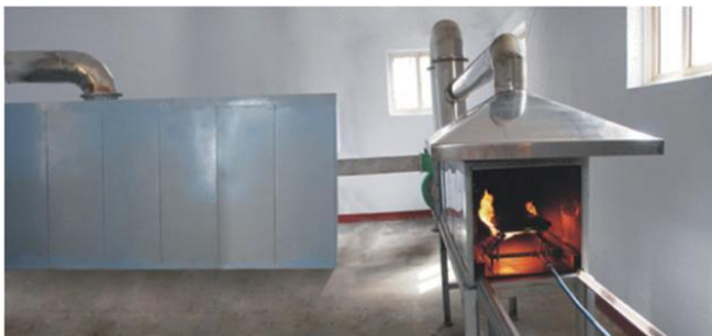
输送带酒精喷灯燃烧性能试验箱 CONVEYOR BELT ALCOHOL LAMP COMUSTION CHAMBER
