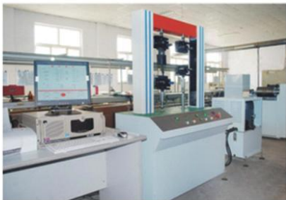
钢丝绳芯胶带动态粘合强度试验机 STEEL WIRE ROPE CORE BELT DYNAMIC ADHESION STRENGTH TESTING MACHINE
