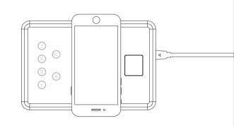
4. USB Wire Charging: Connect the device with the USB Input Port of the Q9 through the USB charging cable.
