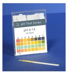
Non-bleeding indicator sticks for rapid reading of weakly buffered or strongly alkaline pH solutions.
