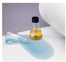
Protective absorbent paper with a plastic backing to absorb small spills and prevent damage to worktops. It makes cleaning up busy labs a simple task by simply replacing the surface covering.
