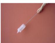
Nylon head brushes with fan shaped end and wire handle for cleaning measuring cylinders.
