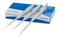
Equipped with a precision digital display, the new line is continuously adjustable down to a very fine volume resolution. Single-handed volume setting is easy and measuring unknown volumes by aspiration is also possible with a high degree of accuracy.
