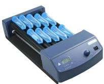
Roller mixers are ideal for gentle mixing at a steady even rate and ideal mixers to prevent sedimentation of samples. They consist of a number of motor driven rollers which rotate at either a fixed or variable speed. When the samples are placed between the rollers in tubes or bottles, they are gently rolled. A rocking action is also applied whereby the rollers are raised and lowered at one end during rolling. This increases the effectiveness of the mixing.
