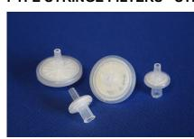
A range of economical, disposable and extremely easy to use PTFE syringe filters. Designed with female luer lock inlet and male luer slip outlets. Sterile filters are RNase, DNase, DNA and pyrogen free and are individually wrapped. Packs of 1000 filters are packaged in clear bags.
