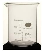
Borosilicate glass beakers with graduations and spout. Range available from 50ml to 3000ml.
