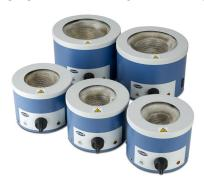
The HM series are a range of controlled heating mantles, available in a range of sizes to accommodate round bottom flasks from 50ml to 1000ml. For added safety, all units feature an emergency cut out which will automatically trigger in the event of a spillage.
