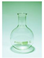
Round bottom, narrow neck, boiling Pyrex flask. Pyrex borosilicate glass offers excellent resistance to chemical corrosion and thermal shock. Complies with ISO 1773 (2000ml flask is supplementary to the ISO range)
