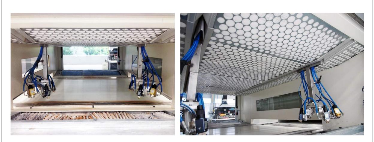
Reciprocal Spray for Coating Flat Substrates in Large Format
