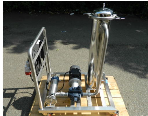
Filter & Pump assembly on Trolley
