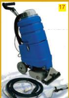
Solution Tank 12 Litres, Recovery Tank 12 Litres Vacuum Motor 1000W 2 Stage 2200mm H2O 50L/Sec Max, Pump By-pass piston type 4 Bar (max) (58psi) 1.5L/Min (Max), Cleaning Width 270mm, Number of jets 3. Cable length 10 metres, Hose assembly length 2.5 metres, Construction Material Expanded polyethylene, Machine Weight 21 Kilograms, Size 280 x 780 x 900mm. Complete with hand tool.
