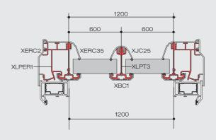
If the roof is to fit to a wall, the effective width of the roof is increased by 30mm.
