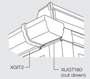
Cut down the XUGT180 to size and clip it onto the eaves beam beneath the gutter stop end.
