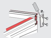
Locate the wallplate end cap, ensure that the shoulder of the cap is sealed onto the wallplate top cap (see above).
