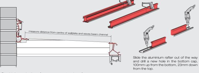
Should the projection of your conservatory be of a non-standard size, then the rafters will require cutting down in length.
