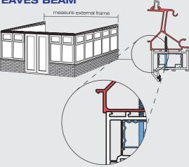
Prior to fitting the eaves beam, run a sealant line along the head of the window. Secure the eaves beam using suitable fixings at 600mm maximum centres, 150mm in from each end.
