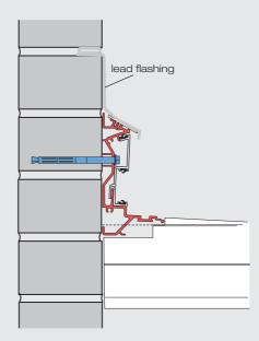
Offer the wallplate assembly to the wall so each end is resting into the notched out firrings. The wallplate should be level.
