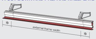
The wallplate assembly should be cut down when the conservatory width is non-standard.
