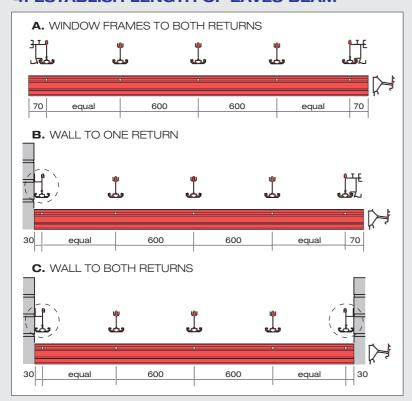
**Note:** the wall end rafter assembly (shown circled above) does not form part of the standard roof kit. This assembly requires ordering separately.
