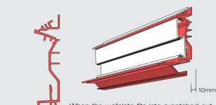
When the wallplate fits into a notched out firring box, the shaded area shown requires cutting away to a depth of 10mm.
