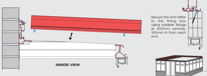
If the eaves beam has been cut down in length then the polycarbonate support trim will need re-cutting and fitting into the eaves beam between the rafters. Ensure that the polycarbonate support adaptors are fitted into each end of the support trim prior to fitting the rafters.
