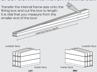
With the box cut to length, the notch details dimensioned below require cutting out of the taller end of the box. Notching is a 2 step approach as shown below.
