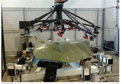
ABOVE: A demonstrator composite winglet structure manufactured automatically as part of a GKN/AMRC project within the STeM programme to reduce assembly times by 30% (GKN photo)
