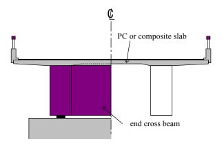
Fig. 2. Two-box girder bridge
