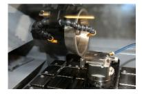
Vacuum system for Precision sectioning / grinding of mounted slides
