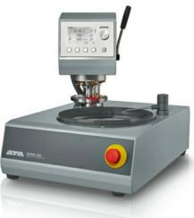
Machines offer both central pressure for clamped samples and also holders for independent loading for maximum flexibility.
