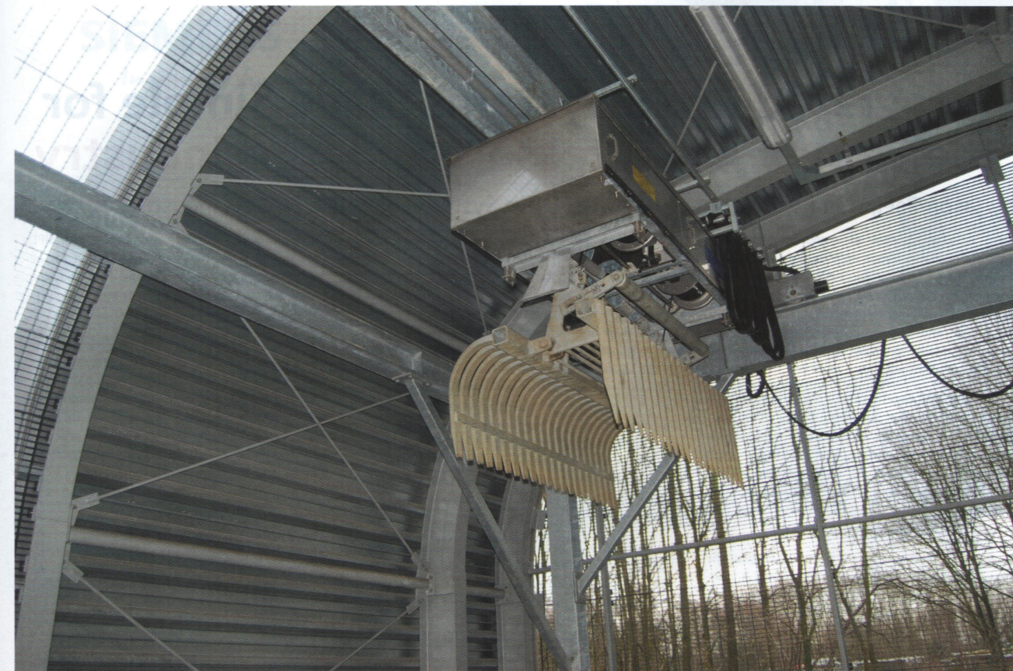
The Bosker system combines a trash rake, overhead conveyor and debris loading system in one
